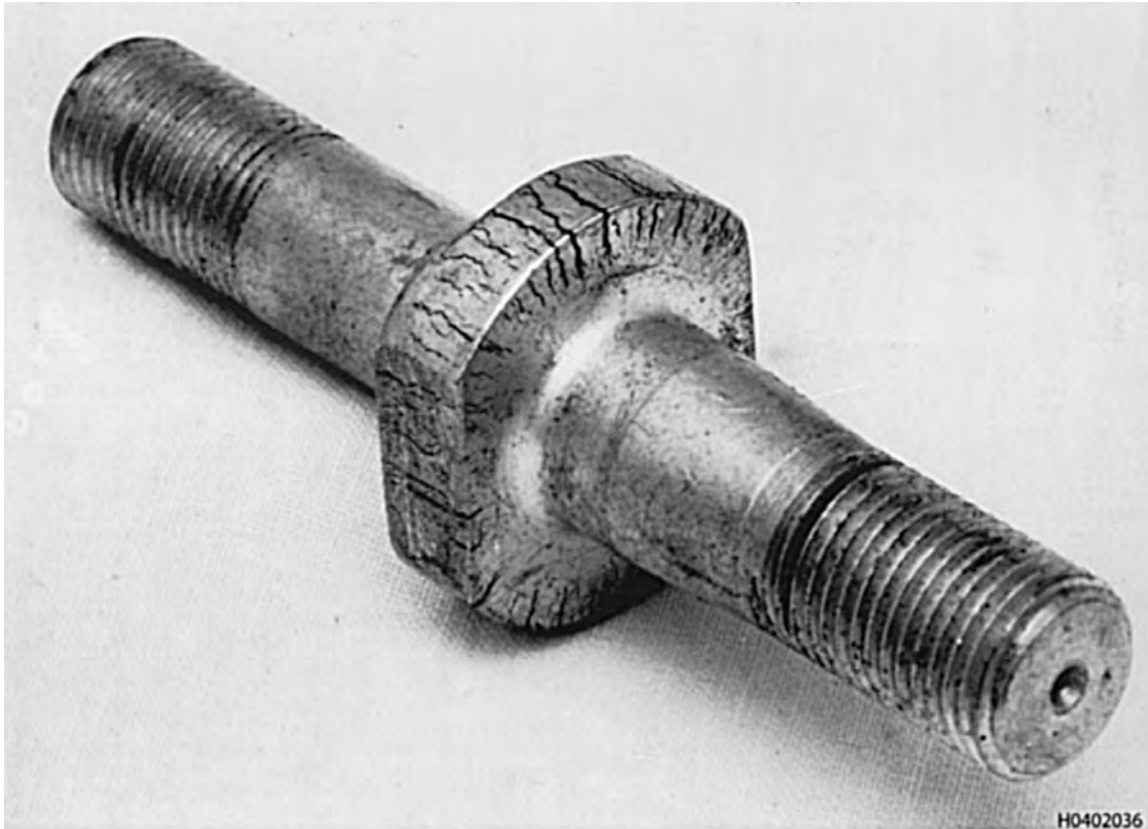
Figure 3-55. Magnetic Particle Indications of Forging Cracks or Bursts in an Upset Section, Severe Case
